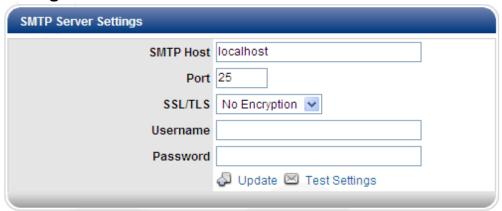
Configuration of the SMTP relay is access under System Tools SMTP Relay.
